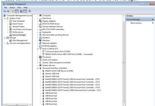
7) Please confirm the installed driver on the screen of the device manager.
