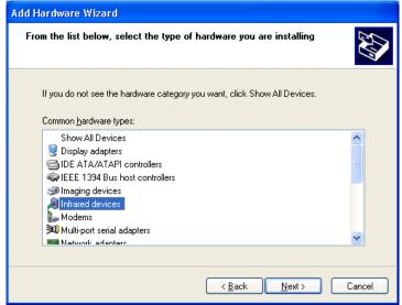
7) Select "Serial Cable using IrDA Protocol" in "(Standard Infrared Port)" and click "Next>" button.
