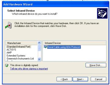
8) Confirm the display of "Serial Cable using IrDA Protocol" and click "Next>" button.
